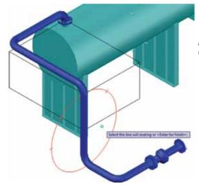
**Auto Route:** (left)\_Multiple options are offered for automatically routing between two points.
